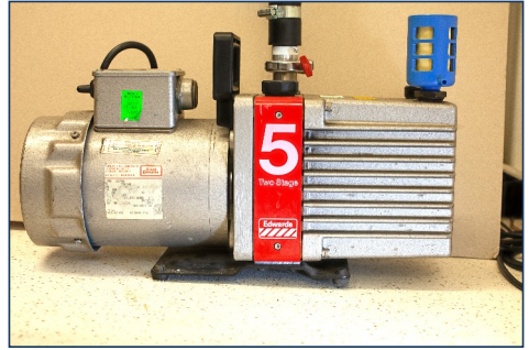
Fig. 4: Reconditioned vacuum pump
