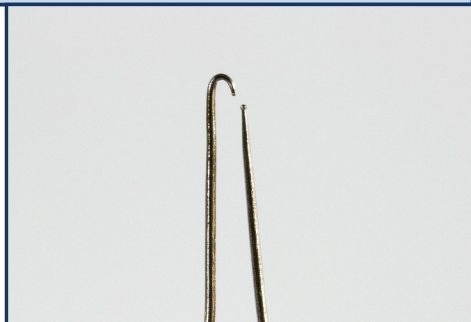
Fig. 2: Detail of Blown Tip of Filament
