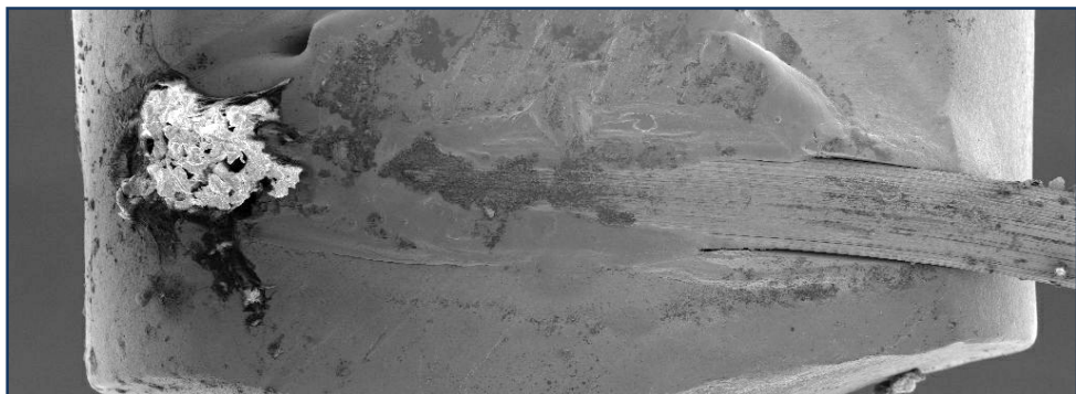
Fig. 8: Foot of a different new filament showing similar manufacturing "artefacts".
