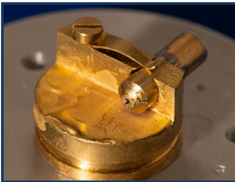
Fig. 4: The Mk II rotating stub holder, showing the rod retained by a spring clip, and the carbon paste coating on the base of the holder.
