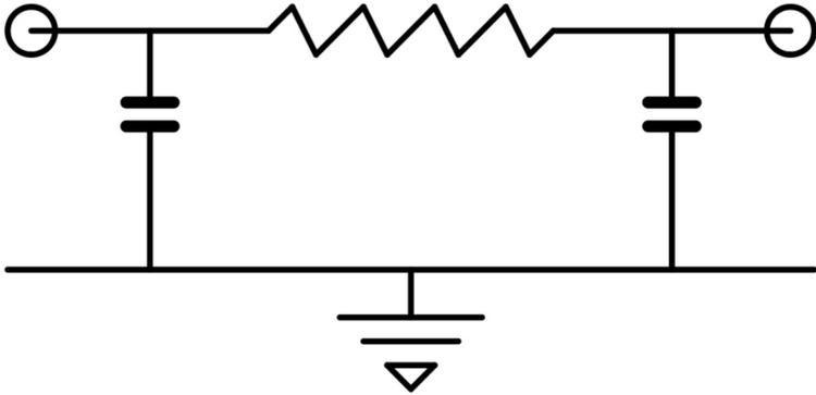
Fig. 1: The circuit diagram of the stage touch alarm “filter”.
