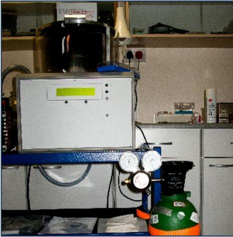
Fig. 2: Sputter coater, with chamber at top, electronics in middle and cylinder of argon at bottom.
